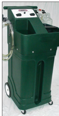
Power steering flush machines like these from Engine Clean Solutions and Wynn Oil Company make the service quick, easy and profitable.
