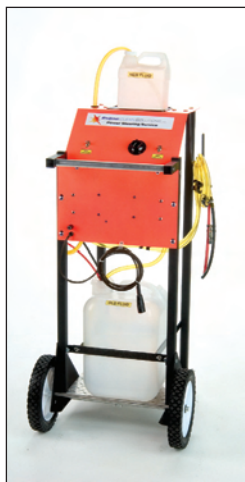
Power steering flush machines like these from Engine Clean Solutions and Wynn Oil Company make the service quick, easy and profitable.
